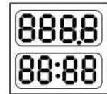
a) All digital of LED display as the right chart when power on. The instrument enters into the initial program with beep.
